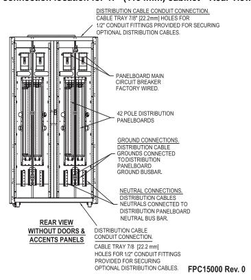
Figure 8 Electrical connection location for 47" cabinet with SqD I-Line panelboard—Front view
